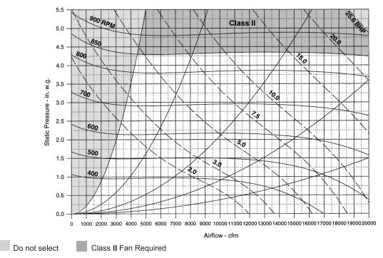
Figure 17: 036C to 040C or RDS 802; 24 in. Forward Curve Supply Fan
