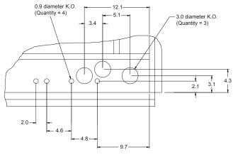
Figure 42: RAH/RDS/RFS/RPS Curb Section A-A
