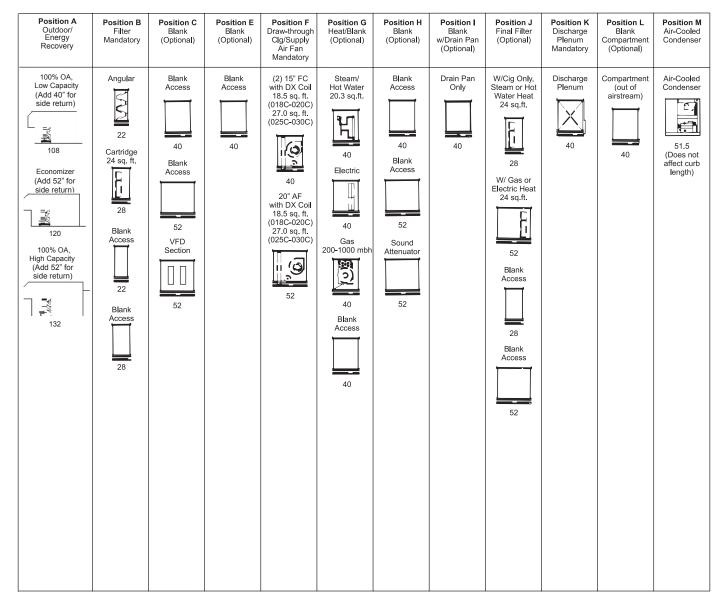
Figure 25: RFS/RPS 015C to 030C, Draw-Through Coil Section (RDS 800 varies slightly)
