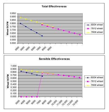
**NOTE:** Based on equal intake and exhaust air flow, minimum purge, and no frost conditions. The 7812 wheel should normally be used if wheel cfm > 8000 cfm.
