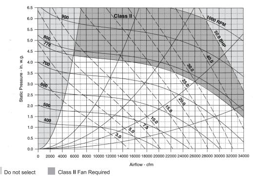
Figure 19: RFS/RPS 045C to 050C or RAH 047C; 27 in. Forward Curved Supply Fan
