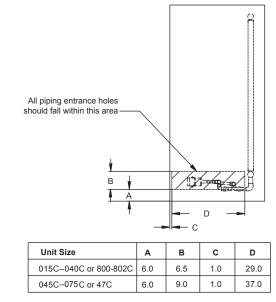
Figure 36: 200 to 1400 MBh Gas Heat/Heat Section
